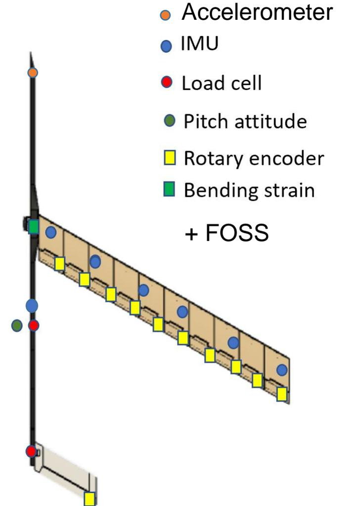
*10 wing TE control surfaces that can be grouped and 1 HTP elevator*
